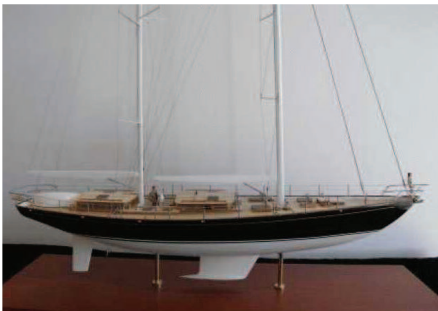
Fig. 7. The hull of this yacht is made from duplex stainless steel 1.4462 and fitted with intelligent anodes.
