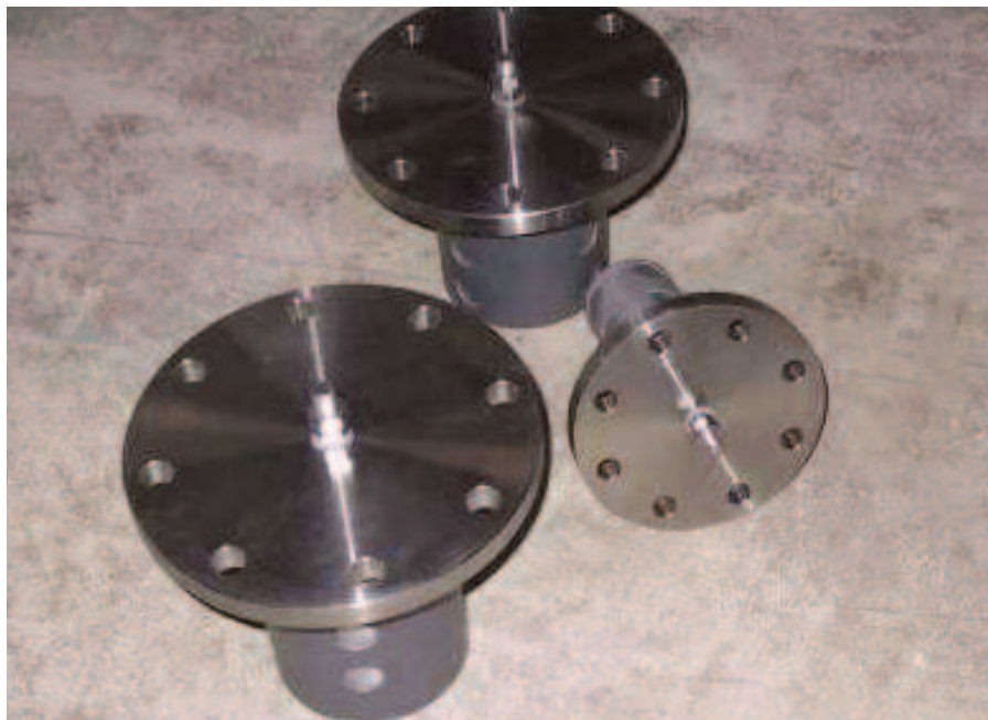
Fig. 4. Corrodium anodes with a stainless steel flange, used for seawater coolers etc. The electronic circuits are built in, eliminating the need for a separate housing or cables (photo by Corrodium B.V.).
