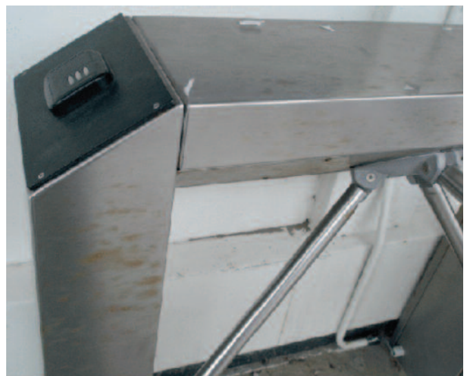
Fig. 11. Turnstile manufactured from stainless steel 316 that has been attacked by aerosols.
